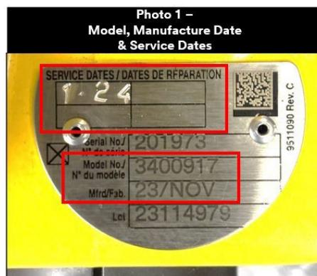
**Step 1.** Locate the model number on the metal identification label (see Photo 1). If your device model number is listed in the table below, proceed to **step 2**. If the model number is not listed below, it is not part of the notice and can be returned to service.
