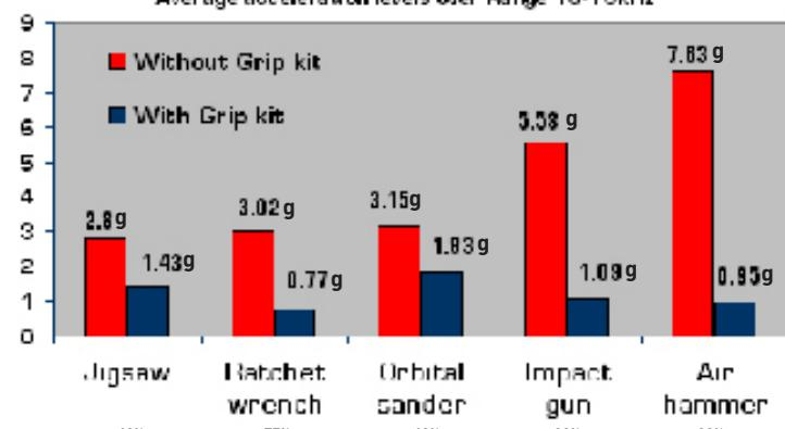
Test show average vibration reductions in a variety of hand tools after an Orthex Grip kit has been applied. Results obtained using Brüel & Kjaer Vibration Meter, Model 2516, for comparison only. Individual test results may vary according to hand size, grip strength, age and manufacturer of tool and other environmental factors.
