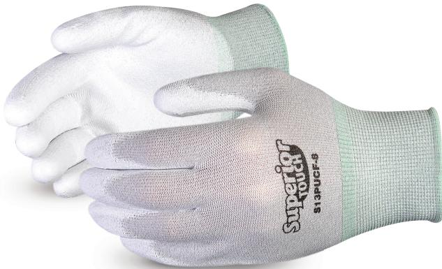
Carbon filament runs throughout the 13-gauge nylon glove body to reduce static build-up on the glove surface for improved performance in electronic applications. Surface resistance (EDS S 11.11) is 107 Ohms at the back of hand, and 109 Ohms on the palm side. These gloves help protect the product from harmful static electricity and are suited for assembling semiconductors, handling compact discs, and handling any electronic products susceptible to electro-static discharge damage.
